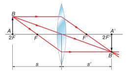
If an object lies at a distance of 2 · f from a converging lens, the image is real, inverted and the same size as the object. It is formed at 2F4 (s4 = 2 · f4).
